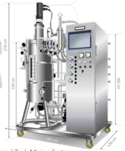
TCICS-100 Stirred Tank Mixing System
