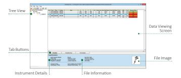
The HAVex meter is supplied with the Vibdata Lite software which allows you to download your measurements via USB for analysis and storage of data as required by the regulations. It is also possible to upgrade to Vibdata Pro which has the following added features:
