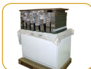
Actual photo during Cabinet Load Testing
