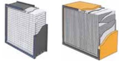
Esco cabinets use Swedish Camfil Farr® mini-pleat filters without aluminum separators to increase filter efficiency, minimize the chance of leakage, and to prolong filter life. Filters include a lightweight aluminum frame for structural stability and elimination of swelling common to conventional wood frames.
