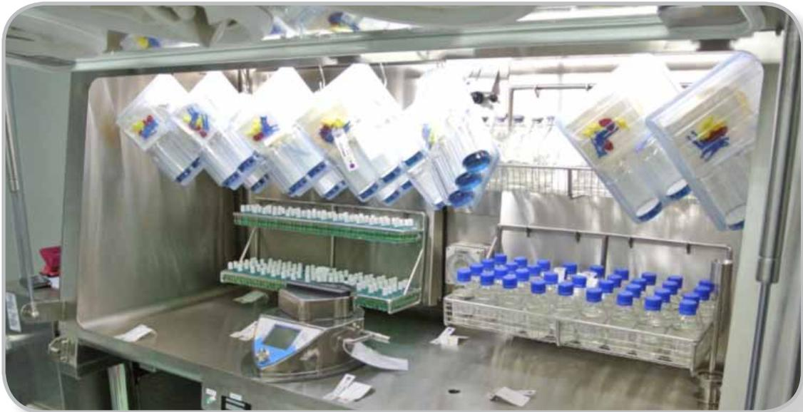
Customized interchangeable racking for sterility test batches
