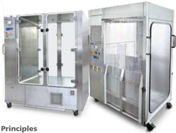
Laminar Flow Horizontal or Vertical Trolleys provide enhanced aseptic work zones by utilizing uni-directional airflow to purge the working environment from contaminants allowing aseptic transfer of materials throughout the Pharmaceutical plant.
